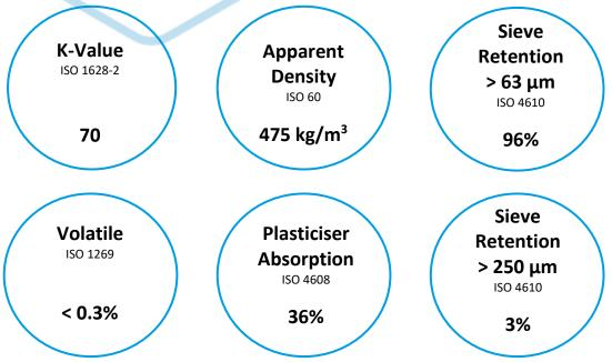
Note: The property data shown above has been obtained from laboratory tests on representative samples of VYNOVA<sup>TM</sup> S7000 polymer. Although the values are typical, they are for guidance only, and must not be used as a basis for specifications.
